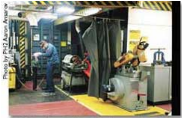
HT I David Brandenburg silver brazes a fitting for a submarine's air bank on board USS McKee .
