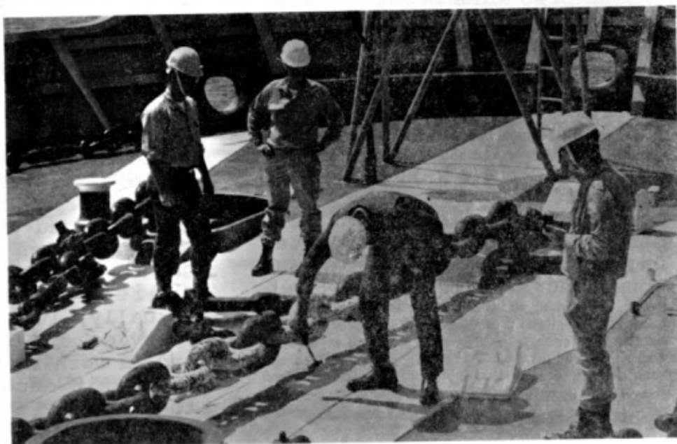
(above) MM2 Coffman removes a lube oil strainer in the Engineroom. (right) CW02 Krzykowski takes the controls in AFT Steering during high speed rudder tests. (below) An INSURV inspector checks a link in the anchor chain during anchoring evolutions on the Forecastle.
