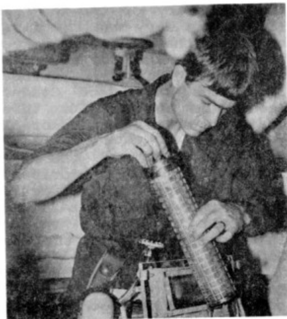
(above) MM2 Coffman removes a lube oil strainer in the Engineroom. (right) CW02 Krzykowski takes the controls in AFT Steering during high speed rudder tests. (below) An INSURV inspector checks a link in the anchor chain during anchoring evolutions on the Forecastle.
