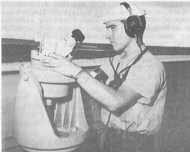
SM3 LYNCH prepares to plot the ship's position by taking land bearings.
